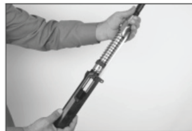
11) Separate the Barrel from the Upper Receiver
