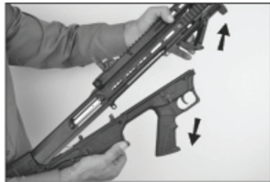
7) Separate the Upper Receiver from the Lower Receiver
